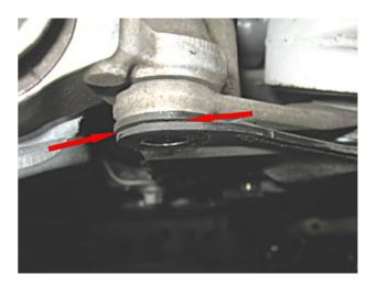
Clean and thoroughly degrease area (use brake cleaner or similar) between two parts of subframe. Blow out any debris etc with compressed air.
