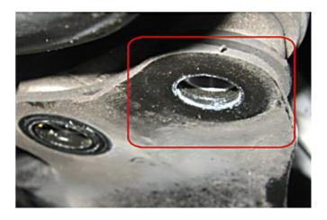
Using a piece of card or similar push a general purpose grease into gap between two parts of subframe.
