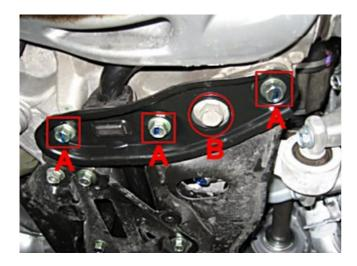
Insert a pry bar or small screwdriver where shown to open gap between the two sections of the subframe.
