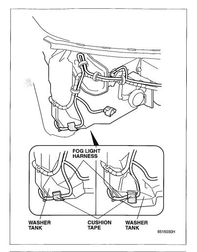
20. Route the fog light harness along the front bumper beam. Install the three clips in the holes in the bumper beam and secure the fog light harness at both ends of the front bumper beam using two wire ties.
