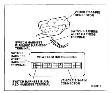
45. Reconnect the vehicle 34-pin connector to the fuse box. Bundle the excess of the switch harness and secure the switch harness to the vehicle harness using a wire tie.
