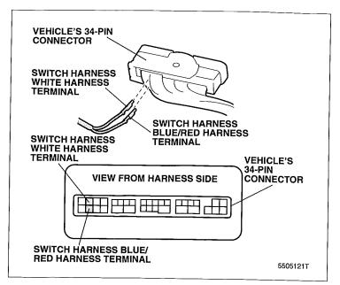
33. Reconnect the vehicle 34-pin connector to the fuse box and secure the switch harness to the vehicle harness using a wire tie.
