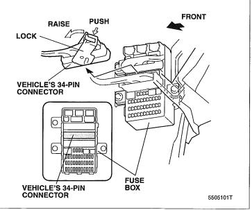
44. Connect the switch harness blue/red harness terminal and white harness terminal to the vehicle's 34-pin connector.
