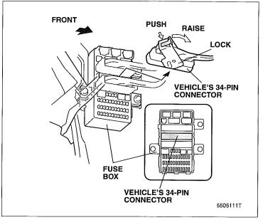
32. Connect the switch harness blue/red harness terminal and white harness terminal to the vehicle's 34-pin connector.
