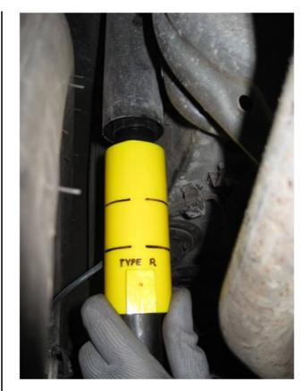
Ensure that depth indication mark on jig (2) is in line with the bottom of the dust cover(1). Fig B. Relevant to the model being treated.
