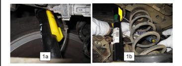
8. Again apply 2 short bursts of lubricant through applicator jig.
