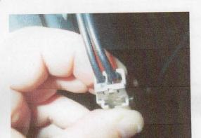
To repair this problem, replace the sub feeder harness, ensuring it is routed correctly.
