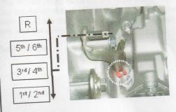
To change gear, the select lever must move forward and downward (this corresponds with moving the gear
