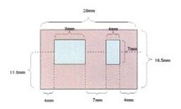
When you have cut out the sections from the EPT sealer place the sealer onto the top off the microphone as shown below.
