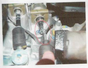
If required replace affected gear change cables with a new part.
